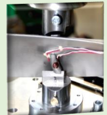
Special force transducer and calibration (Waterproof application with strain gage)
